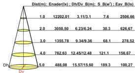
Beam Angie (B): H114.6 V114.7 Field Angle(F): H155.4 V155.1
